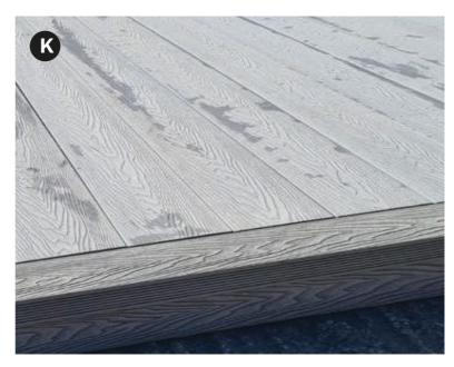
Ezydecking composite decking will lighten and lose up to 30% of its original colour. It can take up to 6 months to stabilise and reach its final colour.
